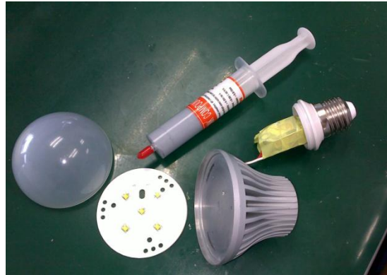
Figure 14: XP-E HEW A21 lamp components
