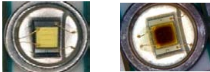
Figure 8: The image on the left is the normal appearance of a chip in an XLamp XP-E LED. The chip in the image on the right has discolored due to exposure to VOCs.
