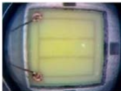
Figure 11: The progression of VOC outgassing from an LEDs silicone encapsulant. This XLamp XP-E LED was exposed to VOCs beneath a secondary optic in a fixture. The volatiles caused the encapsulant to discolor and block the light being emitted from the LED. The optic was removed from above the LED, and it was operated for three days. Each day more of the VOC contaminant outgassed from the LED until it was clear.
